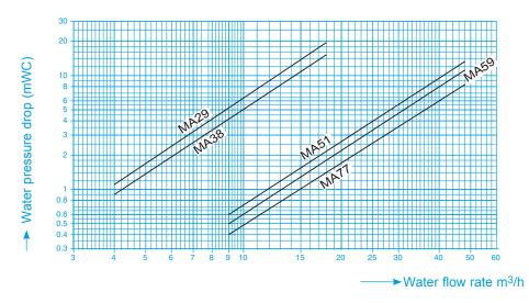
Operating pressure of the Aquatherm module accelerator pump (between the heat pump and the module)
