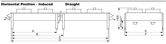
Unit shown has 2 fan lines - no. of motors between the feet is not contractually binding
